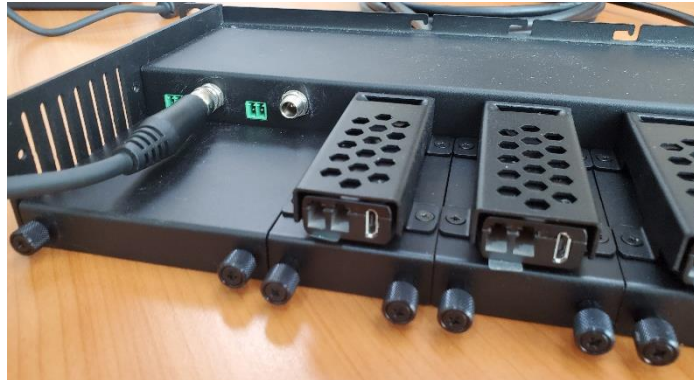
Fig. 6: Mounting the Module bracket on BR-500.
