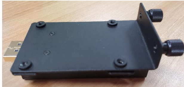
Fig. 3: Module inside the bracket and the slot, two screws are tightened.
