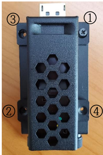
Fig. 4: Holes to insert the screws
