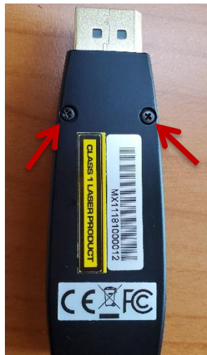
Fig. 1: Remove two screws on the back side of the DisplayPort module
