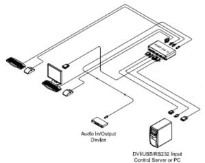
Figure 2– Connection of Transmitter
