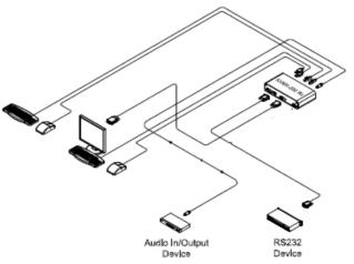
Figure 3- Connection of Receiver
